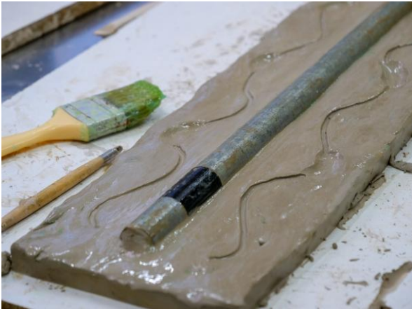
Fig. 47 Clay layup of pipe to create negative for sprue production
