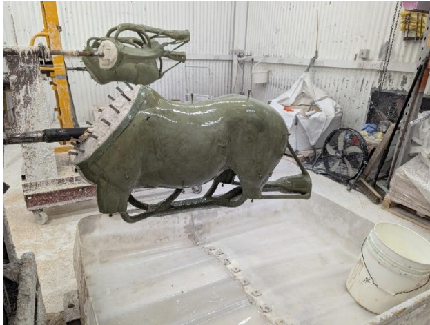
Figure 5 Charlie Langton Horse casting, green casting wax, plaster nails
